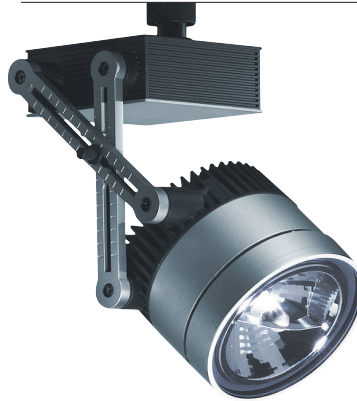
XENO M 1/100 W QR111 halogen spotlight (Order no. 60 711 692), the luminaire can be dimmed via a potentiometer
